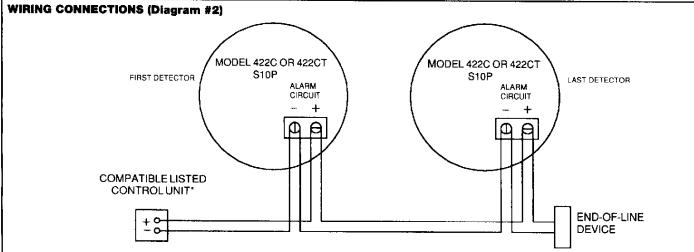
\*ESL 1500 Series Control unit with BMB, ZEM Styles B or D wiring. Maximum line resistance = 100 ohms. Compatibility identifier is C01. Compatible Detectors are ESL Models 422C, 422CT: Compatibility identifier S10P: Maximum 40 detectors per circuit.
