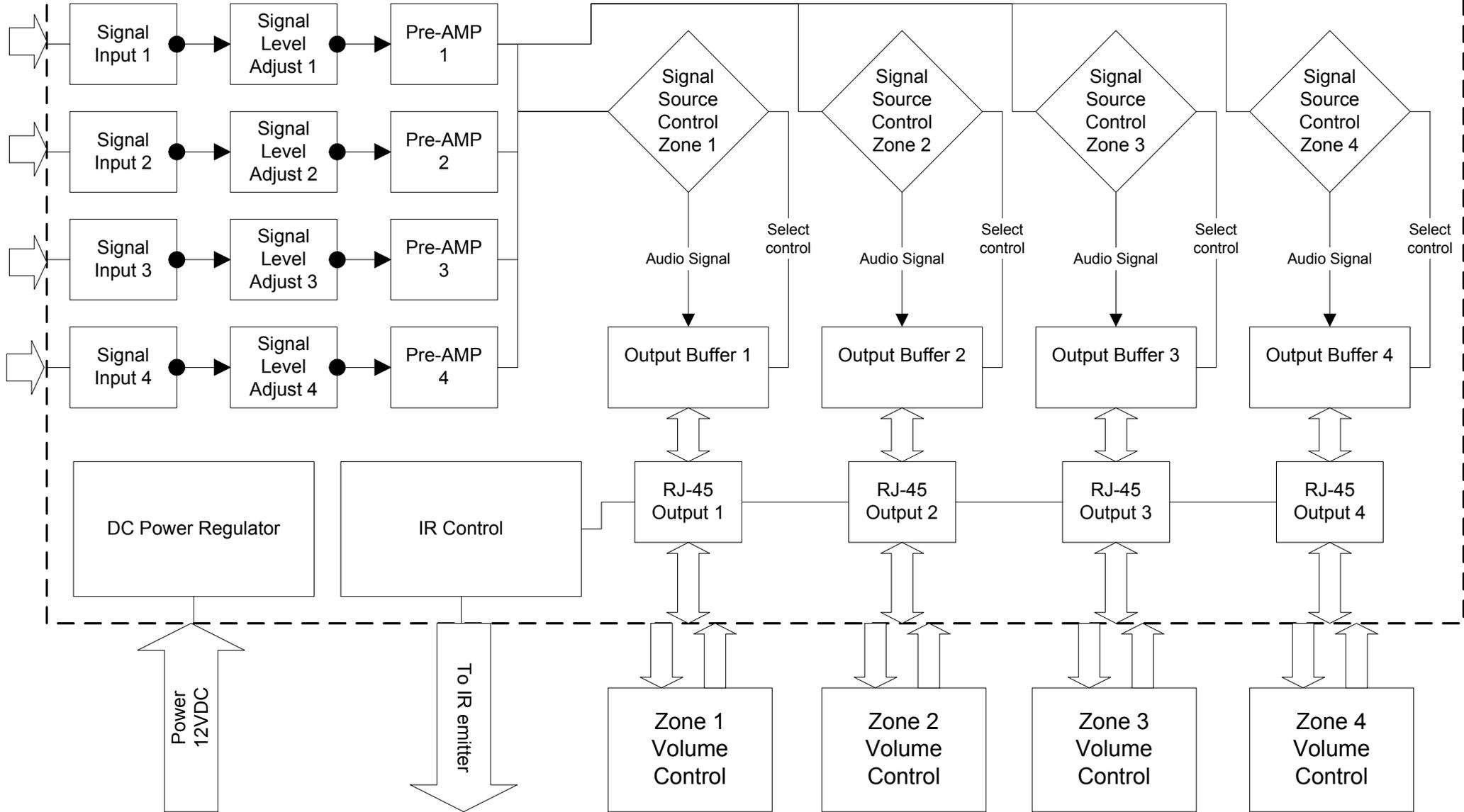
CC-AV1001 Analog 4 Zone Volume Control Block Diagram
