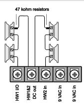
**Note:** Do not install the resistor at the panel terminals. This does not provide supervision of the wire.
