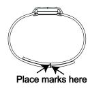
Align the band so the ends of the band are even. Cut the band in the center of the two marks as shown below.
