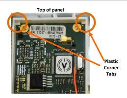
Make sure the module is BELOW the two corner tabs.
