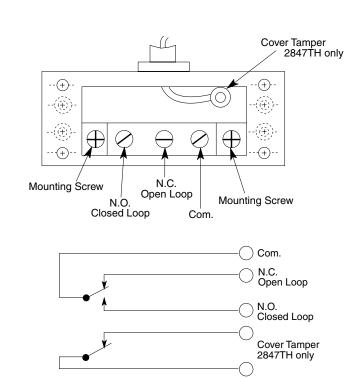
\*Cover tamper wires may be connected in series with closed loop or they may be connected to a separate 24-hour loop.
