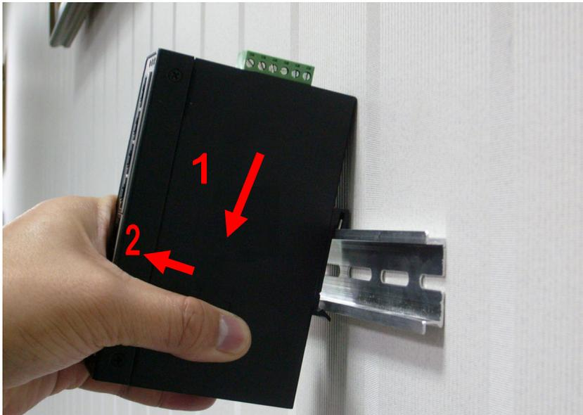
4. Lightly press the bottom of DIN-Rail connector mount to remove it from the track.
