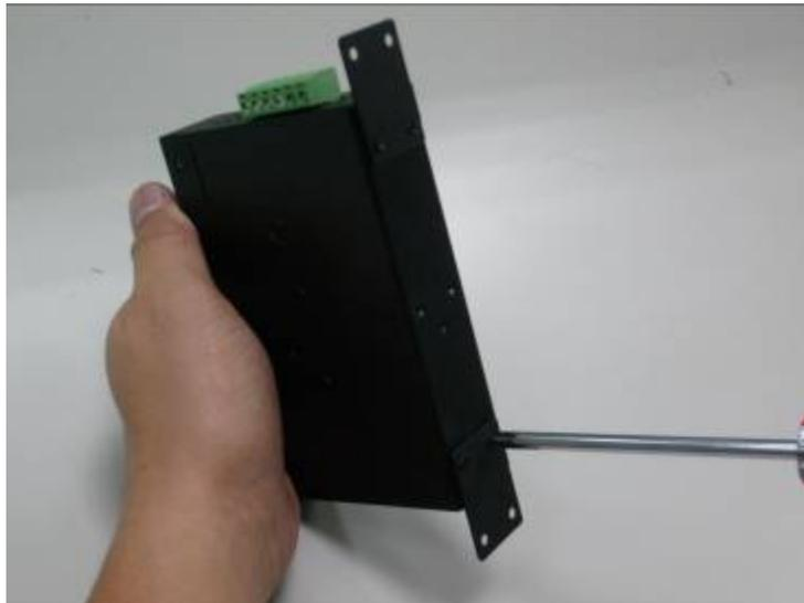
3. Assemble the wall mount plate on the MC355-1T/1S.
