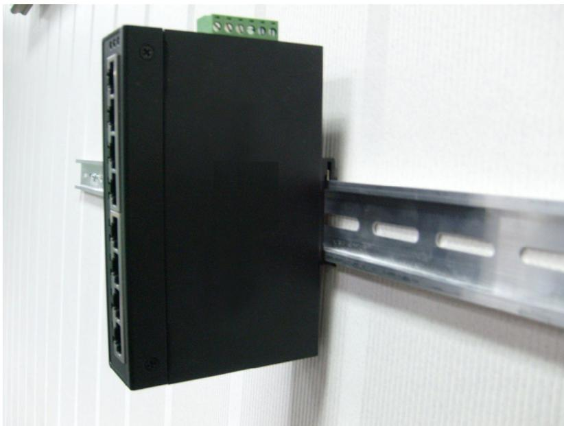
2. Check that the DIN-Rail connector mount is tightly mounted on the track.
