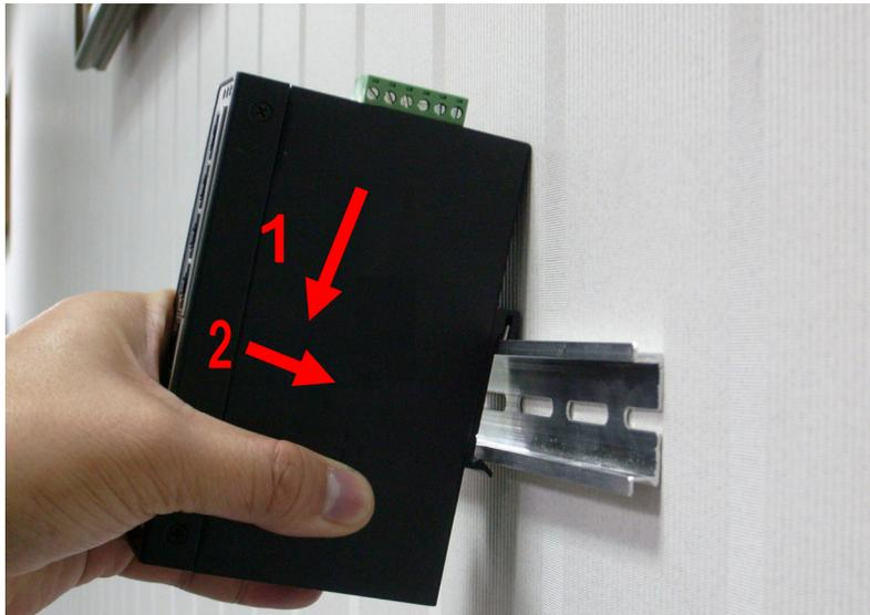
1. Lightly press the bottom of the DIN-Rail connector mount into the track.
