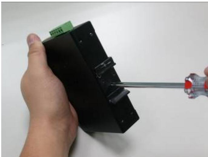
2. Place the wall mount plate on the rear panel of the MC355-1T/1S.
