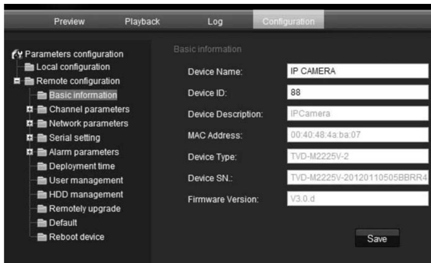
Figure 8: Remote configuration panel (Basic information menu selected)
