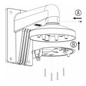
6. Route the camera cables through the inside junction box, align the "FRONT" marks located on the inside of the junction box with the marking on the adapter plate, and then secure the junction box to the adapter plate by tighening the three torx screws.
