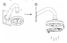
Route the camera cables through the junction box, align the "FRONT" marks located on the inside of the junction box with the marking on the adapter plate, and then secure the junction box to the adapter plate by tightening the three torx screws.
