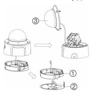
Screw the cup base onto the swan neck mount and tighten with the locking screw, as shown below (A). Attach the camera adapter plate to the cup base (B) using screw A, route the camera cables through the adapter plate.
