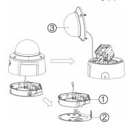
5. Screw the cup base onto the wall mount and tighten with the locking screw, as shown below (A). Attach the camera adapter plate to the cup base (B) using screw A, routing the camera cables through the adapter plate.
