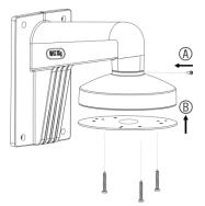
Rotate the trim ring counterclockwise to remove it from the camera. Attach the camera base to the adapter plate using the screws provided with the camera.
