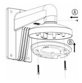
5. Mount the camera base to the adapter plate using the mounting screws M4 × 8 (3 pcs.).
