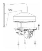
6. Reattach the bubble assembly to the camera base.
