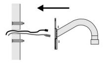
Using the four A screws, attach wedge adapter plate to the cup base.
