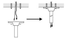
3. Using four screws that are included with the wedge camera, attach the wedge adapter plate to the cup base. Screw the cup base onto the pendant mount and tighten with the locking screw.
