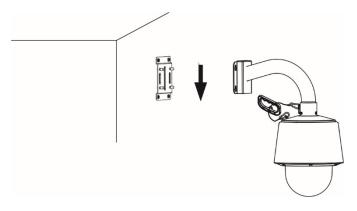
Use the nut and washers A to secure the wall mount to the mounting plate.
