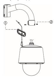
8. Attach the wall mount to the mounting plate, by sliding the mount into place, as shown below.
