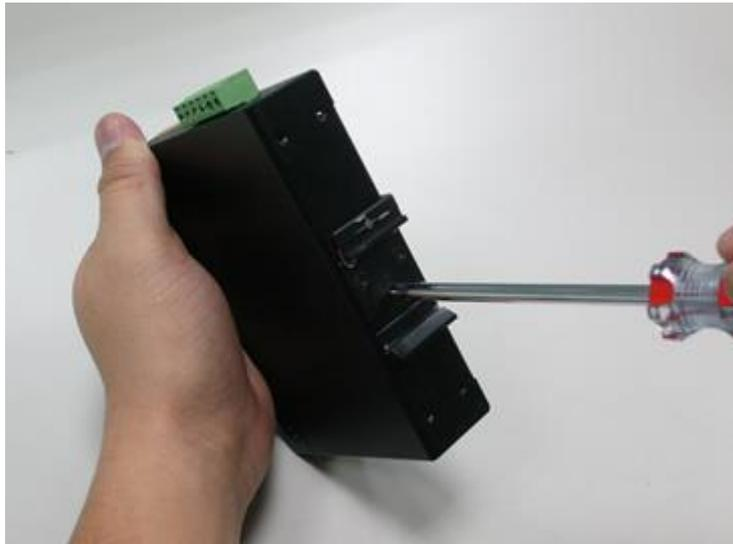
2. Carefully slide the DIN-rail into the track.
