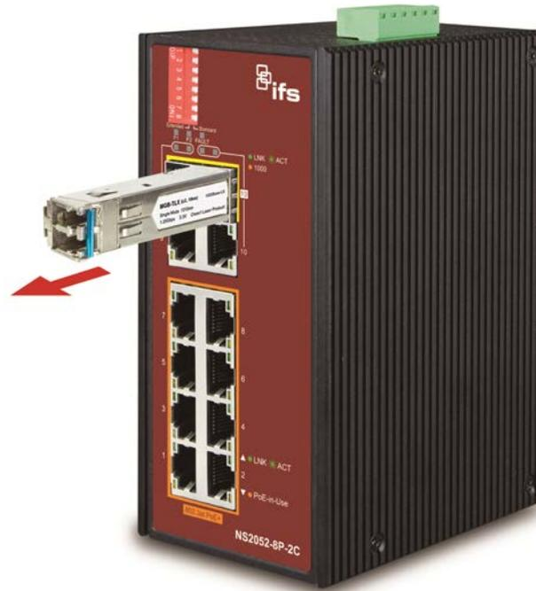
**Note:** Never pull out the module without making use of the lever or the push bolts on the module. Removing the module with force could damage the module and the SFP/SFP+ module slot of the industrial PoE+ switch.
