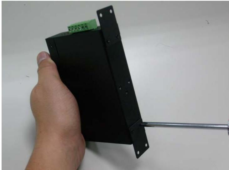
3. Use the screwdriver to screw the wall mount plate onto the industrial PoE+ switch.
