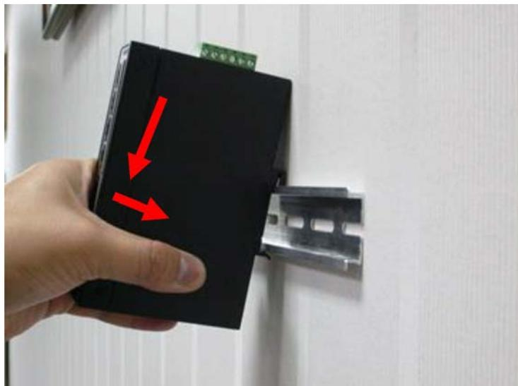
3. Ensure that the DIN-rail is tightly attached to the track.
