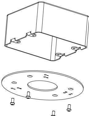
B screws into holes 2 or B screws into holes 1. Refer to the *Supported equipment* section.
