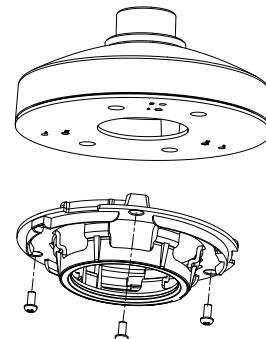
3. Make the proper connections to the camera harness and conceal the cables. Reattach the camera body to the base and adjust the position of the lens.
