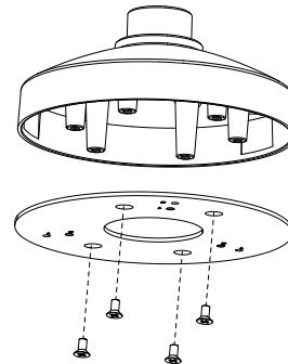
2. Remove the camera body from the turret camera base. Attach the base to the turret adapter plate by inserting the B screws into holes 2 or B screws into holes 1. Refer to the *Supported equipment* section.
