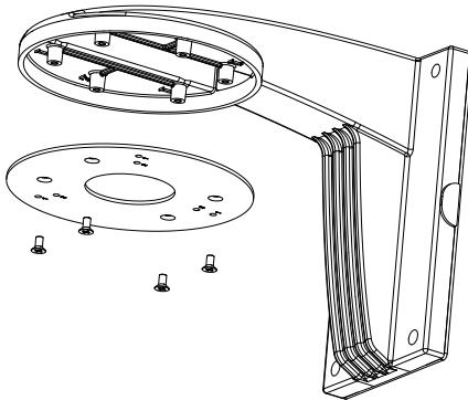
2. Remove the camera body from the turret camera base. Attach the base to the turret adapter plate by inserting the B screws into holes 2 or B screws into holes 1. Refer to the *Supported equipment* section.
