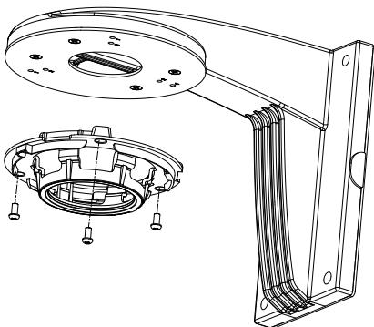
3. Make the proper connections to camera harness and conceal the cables. Reattach the camera body to the base and adjust the position of the lens.
