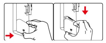
Plug the RJ45 Ethernet cable into the PoE LAN Port of the WMC251-300. Then, slide back the cover of the WMC251-300 to finish the installation.
