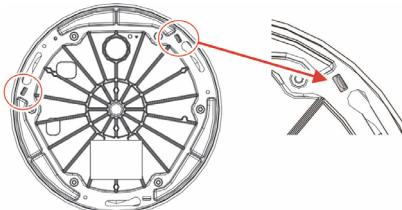
3. Grasp the opening on the side of the cover (1), and pull the cover and base apart to open the camera.
