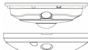
**Note:** When the TruVision 360° camera is mounted to the wall or ceiling, you will not have access to the two clips. In such situations, use a flathead screwdriver to gently pry the cover (see step 3 A.1) apart from the camera base.
