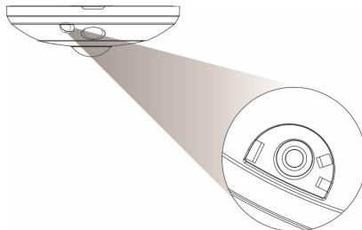
2. Two clips on the cover ring lock it on to the camera base.
