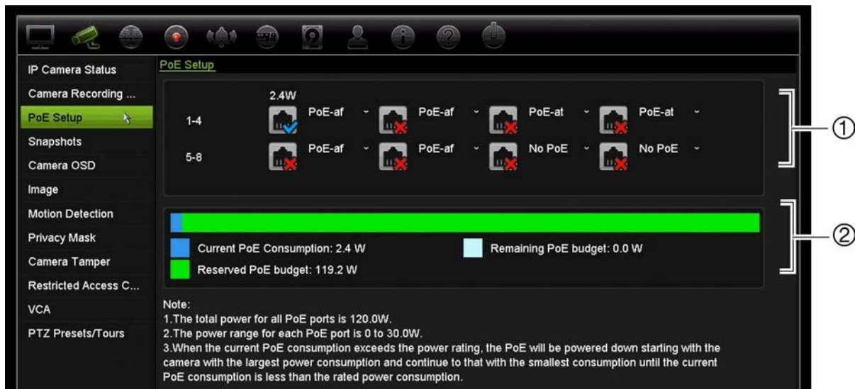
Figure 20: PoE power budget information on IP cameras
