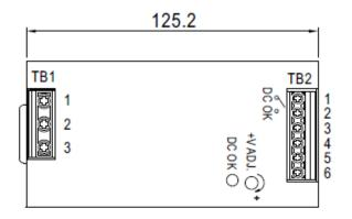
Attach wiring 14 AWG on to proper connections See terminal assignments below:
