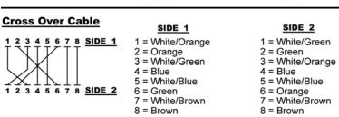
Please make sure your connected cables are with same pin assignment and color as above picture before deploying the cables into your network.
