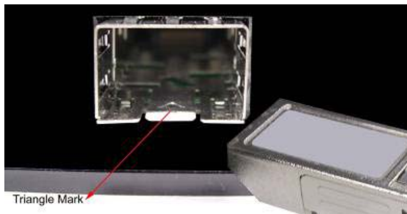
Figure 2-19: Plug-in the SFP transceiver
