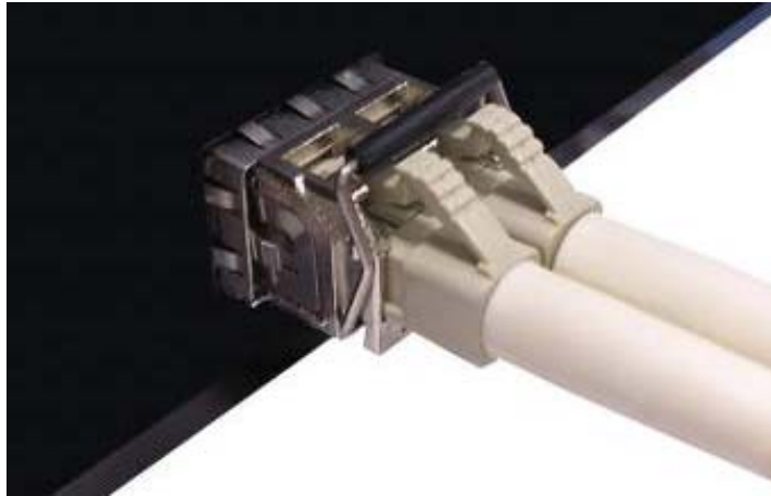
Figure 2-20: LC fiber optical cable connects to the transceiver
