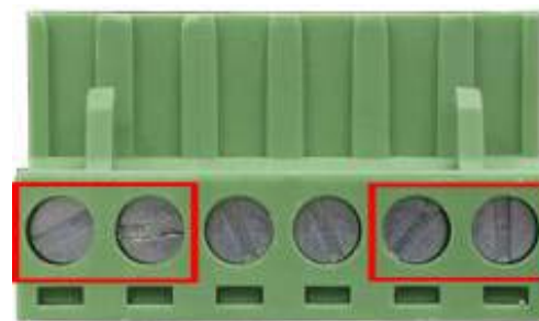
Figure 2-15: Wiring the redundant power inputs
