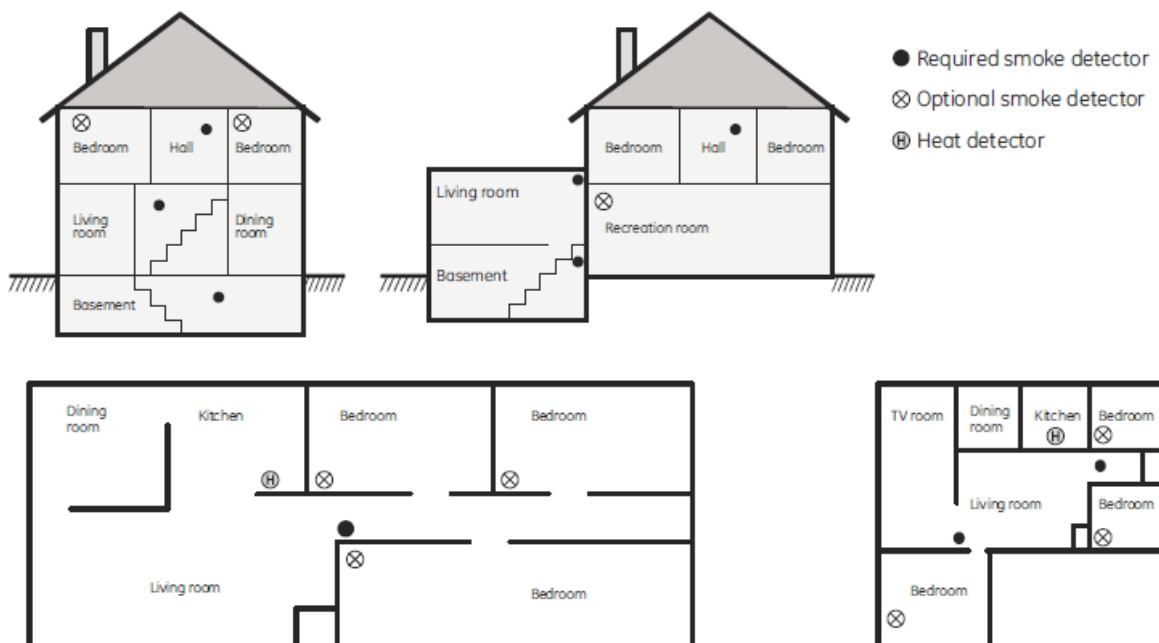
Figure 2. Smoke and Heat Detector Locations:
