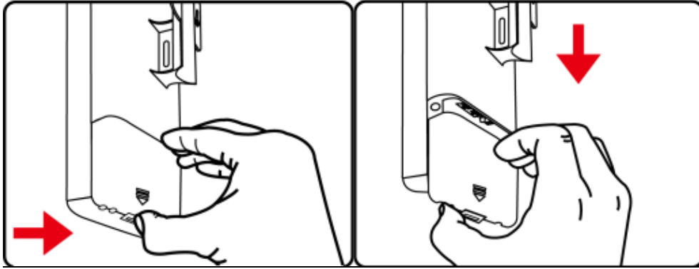
Figure 3-1 Connect the Antenna
