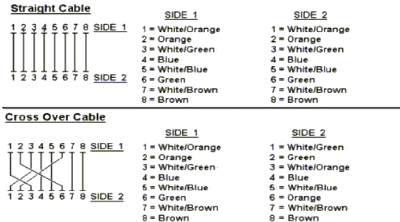
Figure A-1: Straight-Through and Crossover Cable
