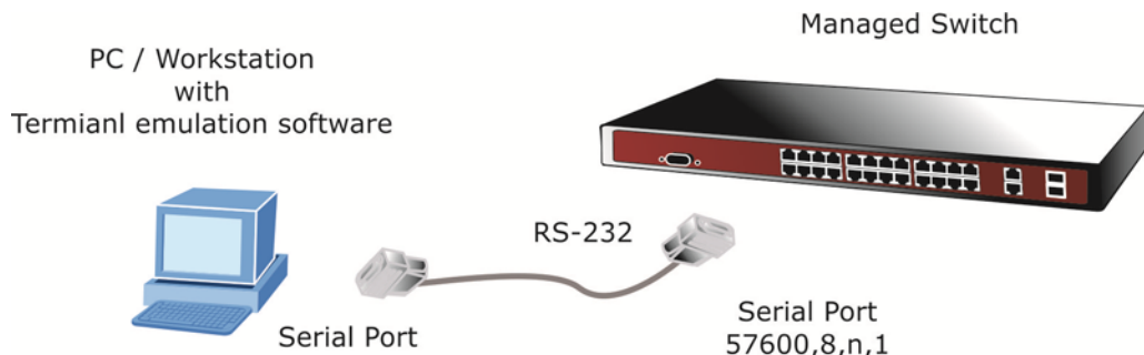
Figure 1: Console Management Diagram
