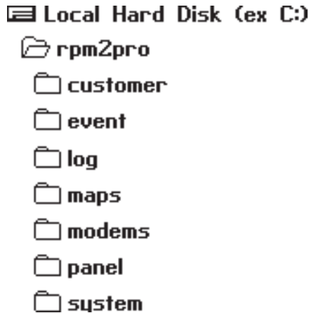
Figure 10.1 Standalone Configuration Directory Structure
