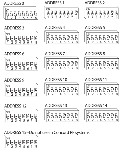
Figure 12: Unit number DIP switch settings
