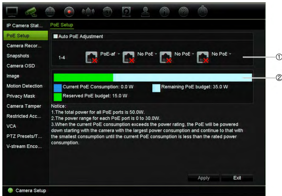
Figure 24: PoE power budget information on IP cameras (4-channel PoE recorder shown)
