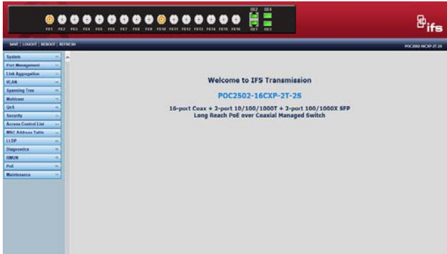
Figure 8: Web Main Screen of POC2502 Managed Switch
