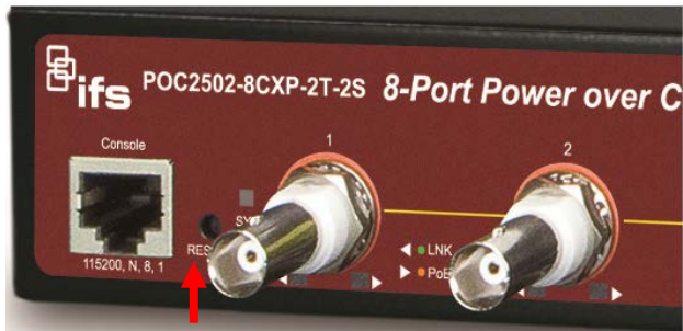
Figure 10: POC2502-8CXP Reset Button
