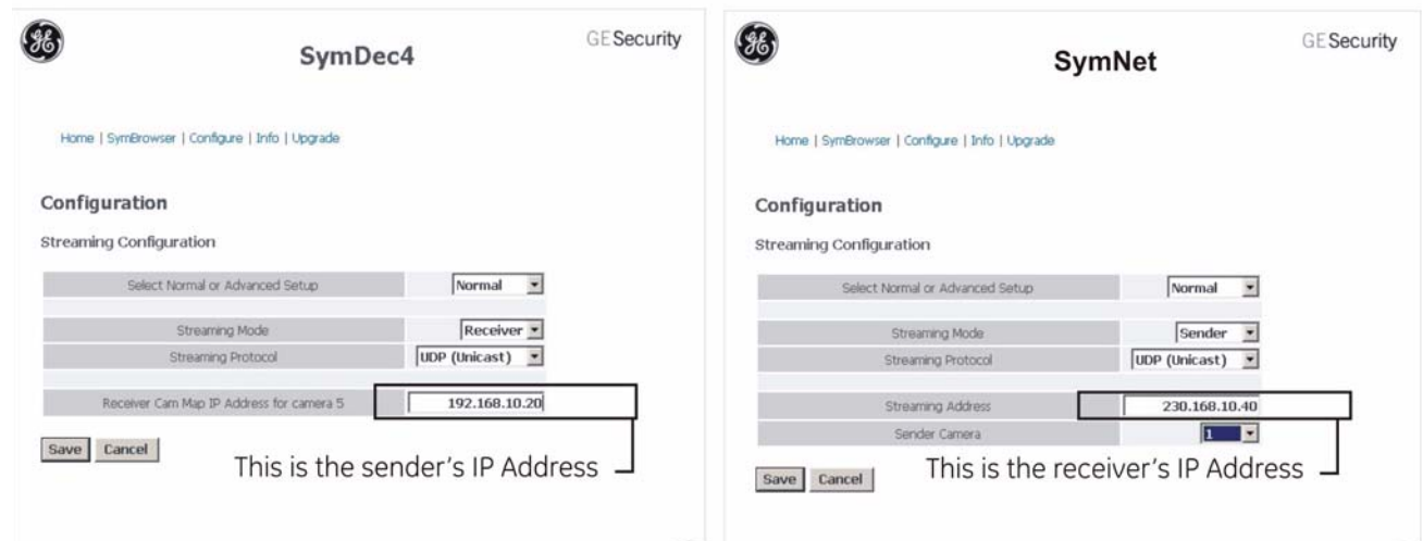
Figure 15. SymDec 4 setup as receiver and SymNet setup as sender
